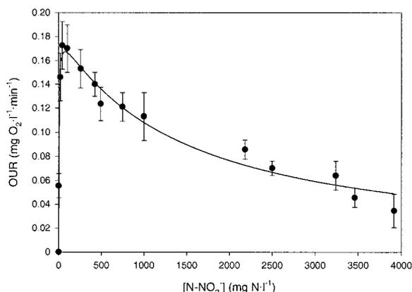
Fig. 2. OUR profile of the nitrite-oxidizing organisms, obtained to nitrite concentrations from 1 to 4000 mg N-NO<sub>2</sub><sup>-</sup> l<sup>-1</sup>. Experimental data (●) and model prediction (—). At pH = 7.5 ± 0.1 and T = 23 ± 1 °C.
