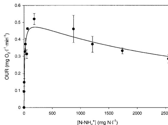
Fig. 1. O<sub>2</sub> uptake rate (OUR) profile of the ammonia-oxidizing organisms, obtained to ammonia concentrations from 1 to 2500 mg N-NH<sub>4</sub><sup>+</sup> l<sup>-1</sup>. Experimental data (●) and model prediction (—). At pH =  $7.5 \pm 0.1$  and T =  $23 \pm 1$  °C.
